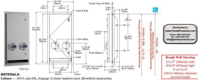
Flange — 18-8 S, type-304, 22-gauge (0.8mm) stainless steel with satin finish. Drawn and beveled, one-piece, seamless construction. Adjustable escutcheon-type flange permits semi- or fully-recessed installation.
