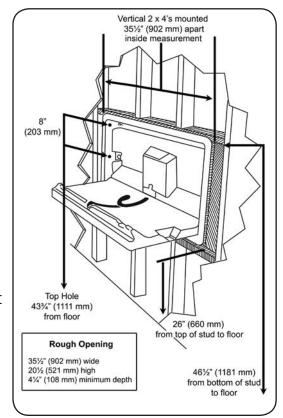
4. Place the unit into the recessed area and insert the screws and flat washers to hold the unit in place. It may be necessary to adjust the level of unit by using a shim on the top right or left side of the unit before tightening securely to the studs.
